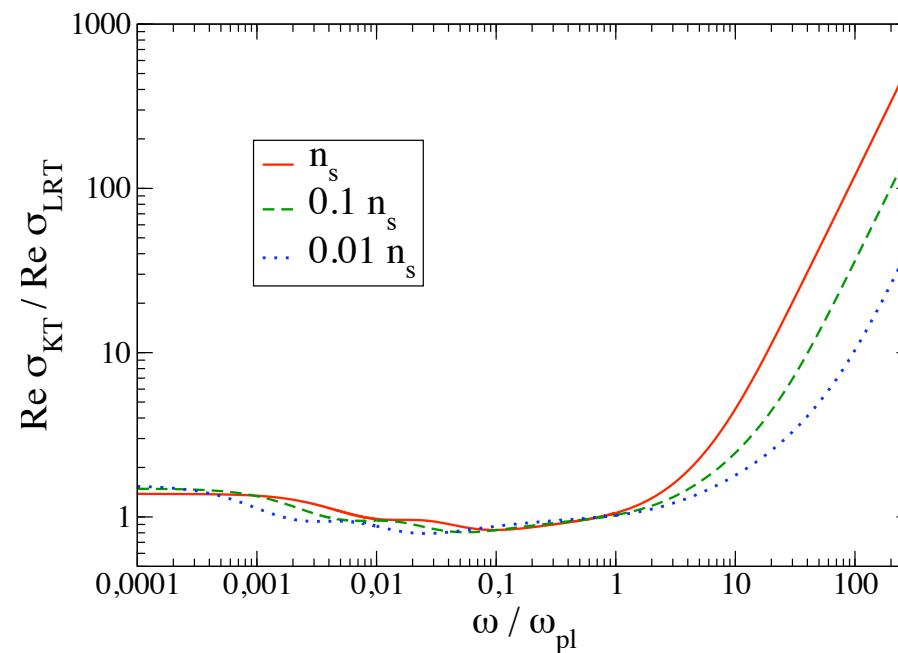
Correction factor  $r^{(2)}(\omega)$  due to higher moments, including e-e-correlations, for static case
